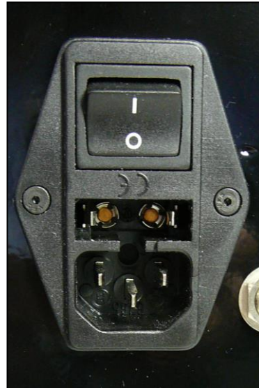
FUSE HOLDER REMOVED
